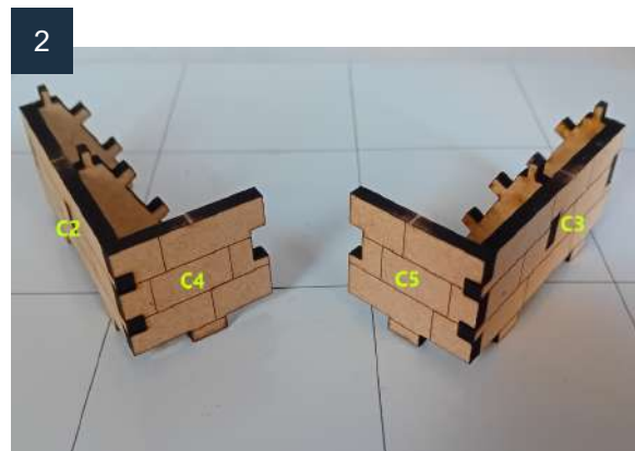
2. Assemble the C4 part to the C2 part. Assemble the C5 part to the C3 part.
