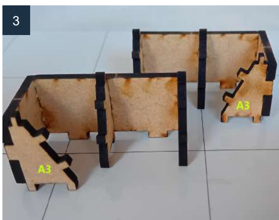
3. Assemble one A3 part on the side of the C4 & C5 parts.
